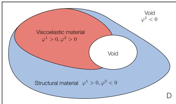
**Figure 2.** Illustration of a multi-material structure defined by two level set functions. The first level set function  $\varphi^1$  determines the placement of material, while the second level set function  $\varphi^2$  distinguishes between structural and viscoelastic material.
