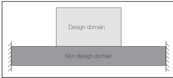
**Figure 10.** The design and nondesign domains for case study II. The nondesign domain is clamped at both sides and cannot be modified by the optimization routine.
