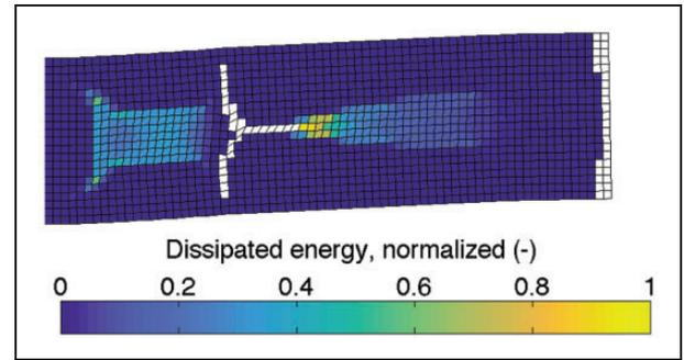
**Figure 8.** The energy dissipated for each element for the first eigenmode of the structure. The values are normalized with respect to the maximum energy dissipated in an element. The obtained result is directly related to the shear strain given in Figure 7a. The uncolored represent void elements within the design.
