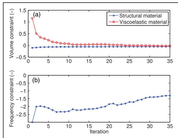
**Figure 6.** The history of the volume (top) and frequency (bottom) constraint values during the optimization. The constraints are normalized with respect to the specified maximum value. Positive values represent unsatisfied constraints.
