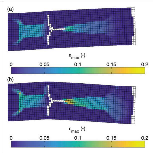
**Figure 7.** The deformation shapes and corresponding maximum shear strain  $\varepsilon_{\max}$  for the first (a) and second (b) eigenmode of the optimized structure. The uncolored elements represent void elements within the design.
