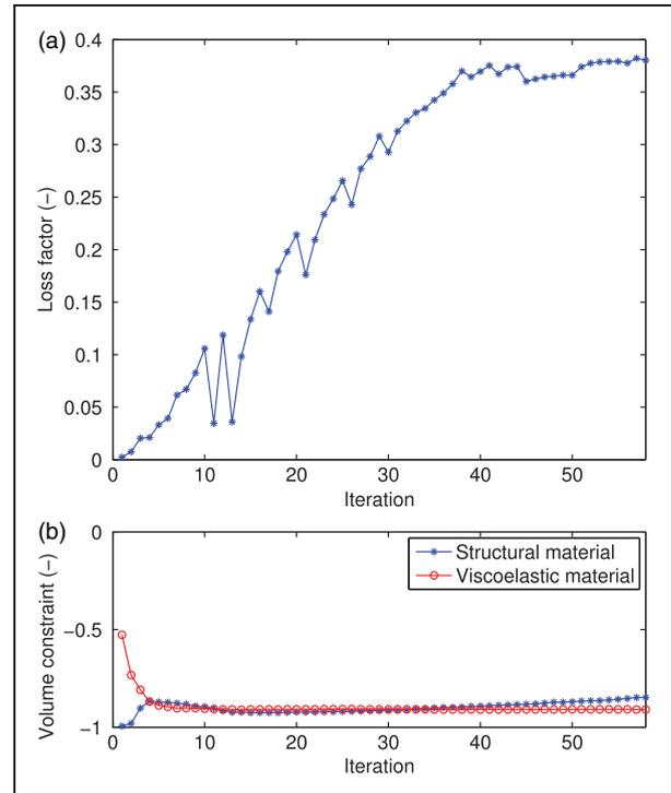
**Figure 12.** The history of the loss factor (a) and normalized volume and frequency constraints (b) during the optimization.
