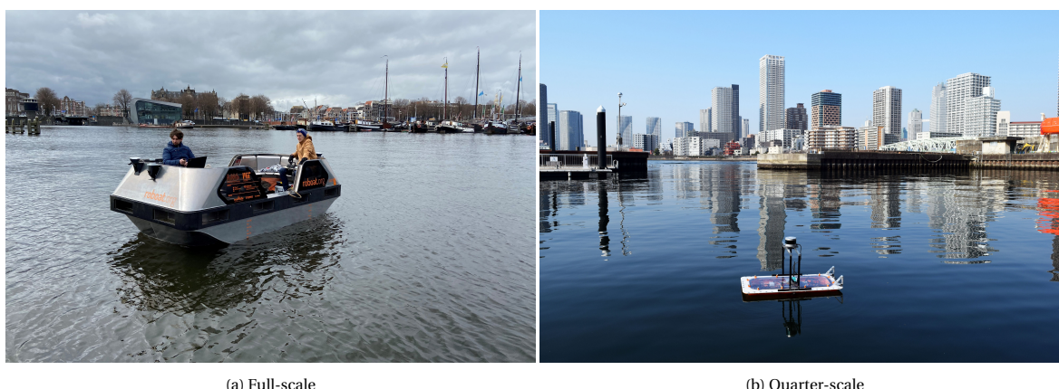
Figure 1.1: Two prototypes of the Autonomous Surface Vessel (ASV) Roboat developed for the Amsterdam canals.
