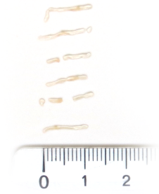
Figure 7.8: Photograph of the result of experiment 3. The figure shows the attempt to obtain a multitude of biopsy samples using an existing biopsy instrument (TruCore II). Six samples were obtained during the experiment, with a varying length between 2 to 15 mm.
