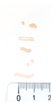
Figure 6.8: Photograph of the result of a preliminary test. The figure shows the attempt to obtain a multitude of biopsy samples through a single insertion.
