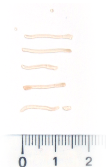
Figure 7.4: Photograph of the result of experiment 1. The figure shows the attempt to obtain a multitude of biopsy samples through a single insertion. Five samples were obtained during the experiment, with a varying length between 10 to 15 mm. One needle cartridge contained no sample.
