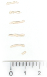
Figure 7.7: Photograph of the result of experiment 3. The figure shows the attempt to obtain a multitude of biopsy samples using the prototype. Six samples were obtained during the experiment, with a varying length between 3 to 11 mm.
