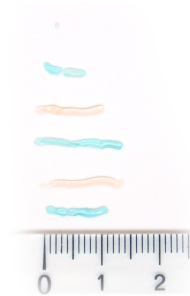
Figure 7.5: Photograph of the result of the first subexperiment of experiment 2. The figure shows the attempt to obtain a multitude of biopsy samples through a single insertion with various orientations. Five samples were obtained during the experiment, with a varying length between 8 to 15 mm. One needle cartridge contained no sample.
