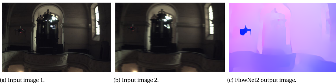
Figure 6.3: Situation in which the MAV is poorly recognizable in the original frames, but much easier to detect in the output of Flownet2. Dataset: MIDGARD [64].
