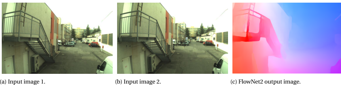
Figure 6.4: Situation in which the MAV is not moving compared to the camera and the MAV is unrecognizable in the output of Flownet2. Dataset: MIDGARD [64].
