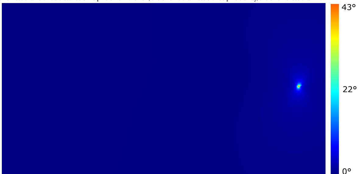
(c) FoE positioned in the right part of the image. 97.0% of the pixels have an error less than 1^\circ , and 99.9% of the pixels have an error less than 5^\circ . At a distance of 28 pixels from the FoE, the error is than less 5^\circ . 137 pixels away, the error is less than 1^\circ .
