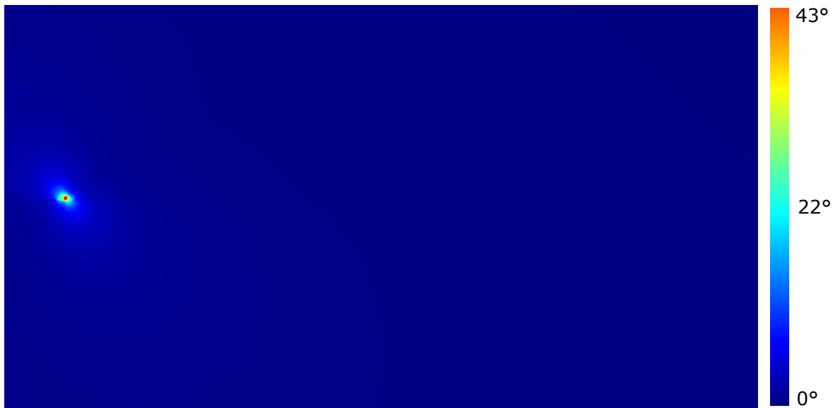
(a) FoE positioned in the left part of the image. 91.4% of the pixels have an error less than 1^\circ , and 99.6% of the pixels have an error less than 5^\circ . At a distance of 52 pixels from the FoE, the error is than less 5^\circ . 232 pixels away, the error is less than 1^\circ .
