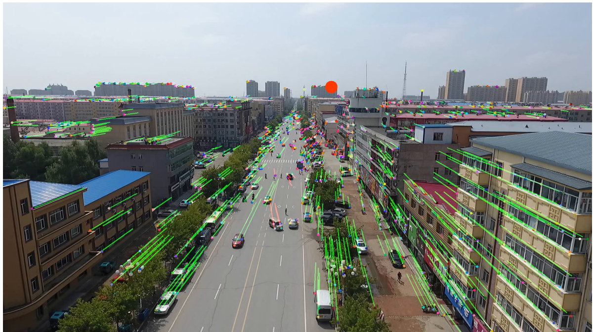
Figure 6.5: Dynamic feature detection using Lucas-Kanade optical flow. The red dot is the calculated FoE. Green lines represent the flow of static features, red lines those of dynamic features. Dataset: VisDrone [70, 71].
