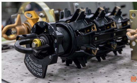
(a) Disconnected tap-changer showing rotary-switch to switch between 5-tap positions from A-E
