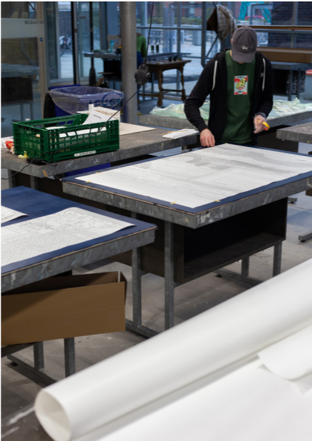
Martino glueing the printed wallpaper on the blue stained plywood panels
