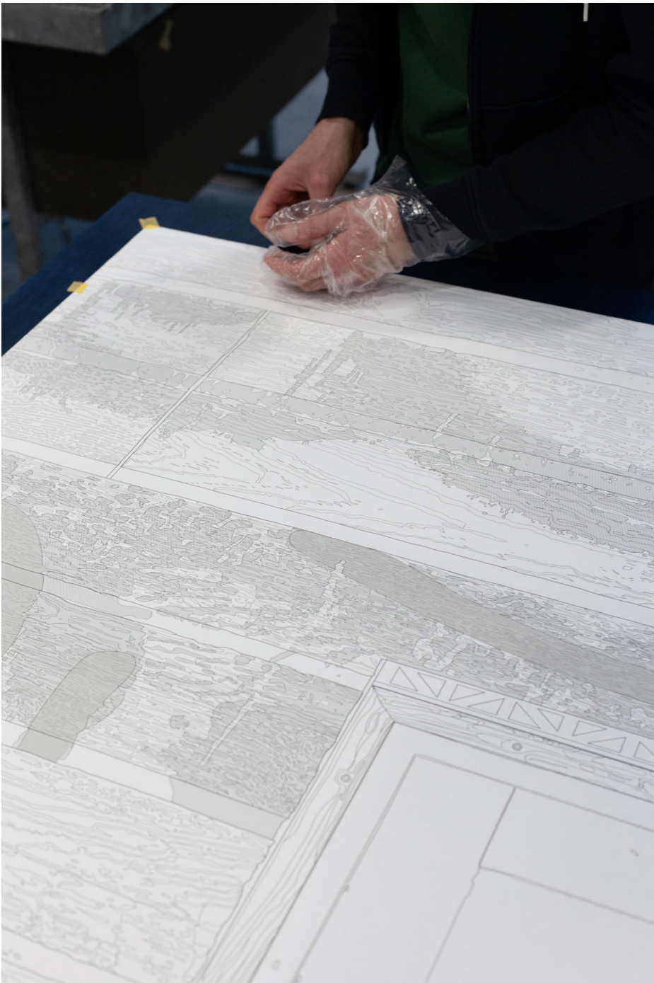
Martino glueing the printed wallpaper on the blue stained plywood panels
