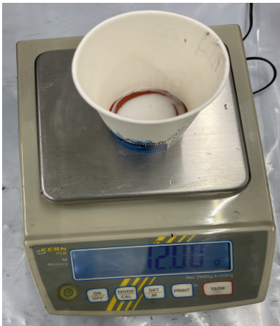
(a) Mixing 6g base with 6g catalyst of TFC Silicon Rubber Type 3
