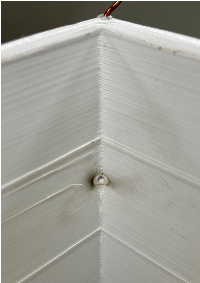
(a) Damage to primary bobbin caused due to repeated core-LV discharges
