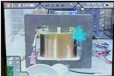
(c) Discharges between ring and core
