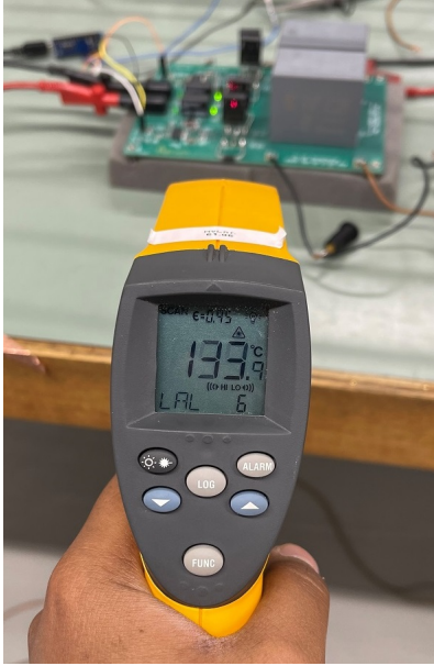
(a) Without any cooling techniques Observed T_{FET}^{max} = 133\text{ }^{\circ}\text{C}
