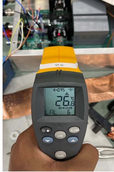
(b) With heatsink and 138 CFM fan Observed T_{FET}^{max} = 26\text{ }^{\circ}\text{C}
