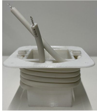
(b) Primary winding made with 25 kV insulated wire. If the insulation is thicker the permittivity of the silicone would increase the C_d by a large factor. Spacing out the wire would improve leakage flux but also causes HV-LV flashovers.
