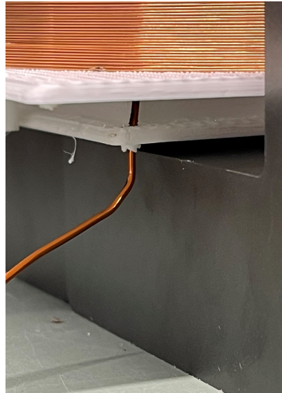
(b) Weak point for flashover at the exit of LV from the primary bobbin
