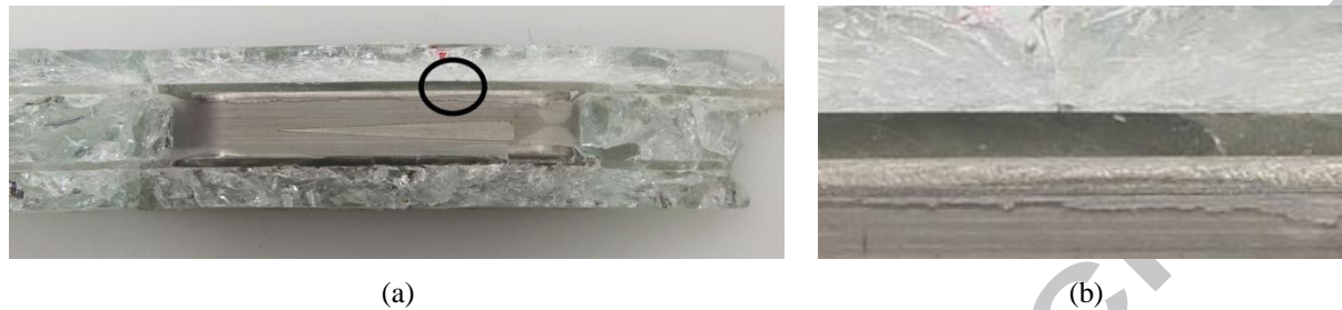
Figure 10. (a) Photo through thickness of the broken glass after testing: failure initiation is indicated by a circle (b) zoom view of the photo at the crack initiation.
