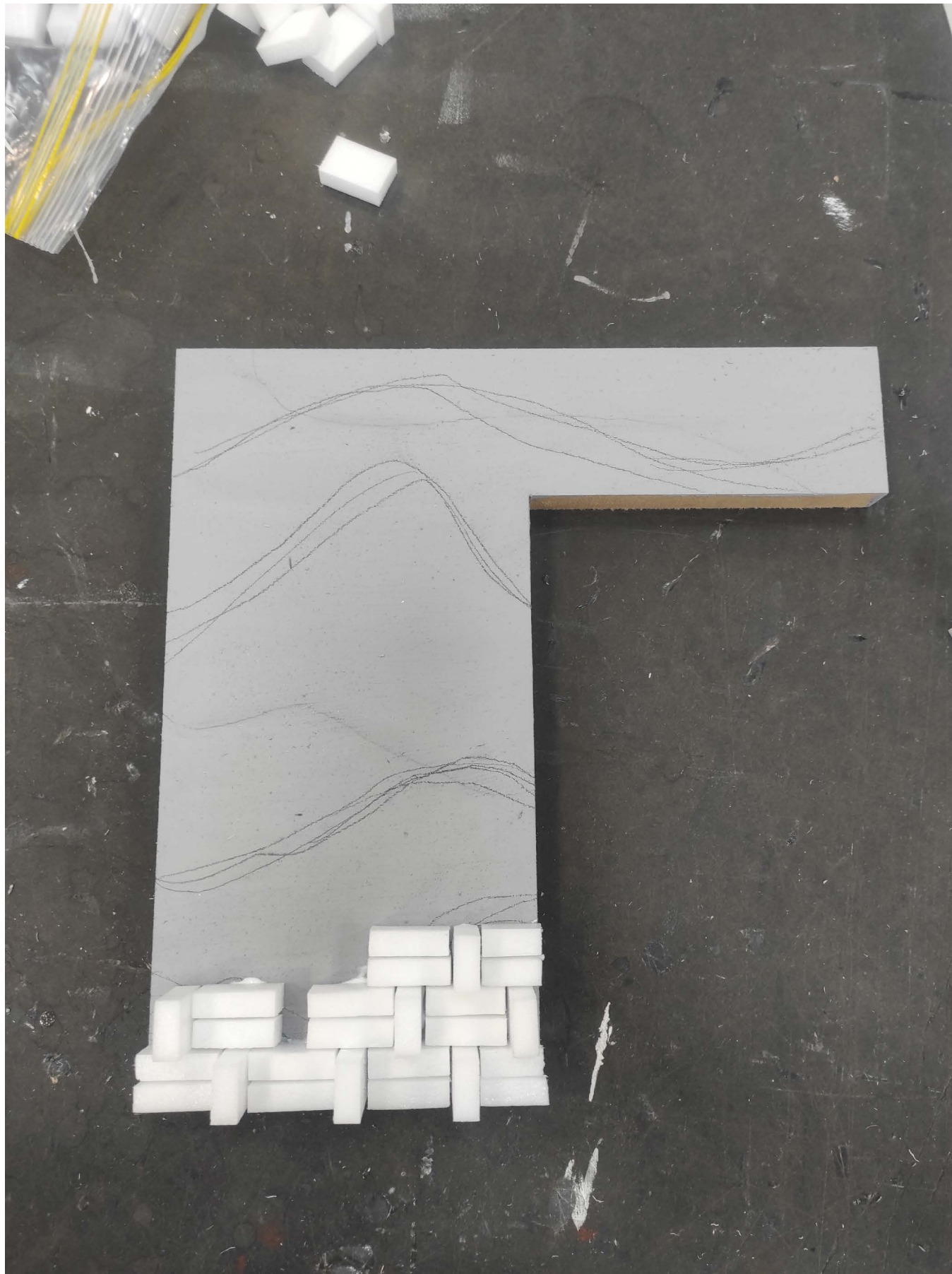
Conceptual 1:10 facade models, building up the facade pattern brick by brick
