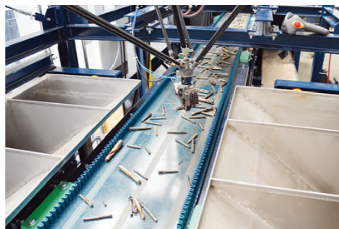
Figure 4: Laser-based metal sorting technology (Cronimet Ferroleg, 2021)
