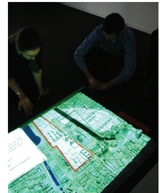
Figure 4: Basic setup of an augmented scale model. First test application for participatory debate about Brussels' Neighbourhood Contracts (source: Stellingwerff & Kuhk, 2004)
