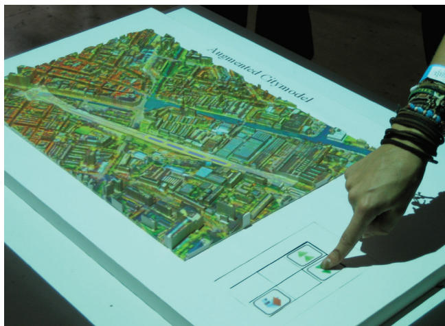
Figure 9: Augmented evaluative model of Railway-zone Delft with interactive interface to choose projected media
