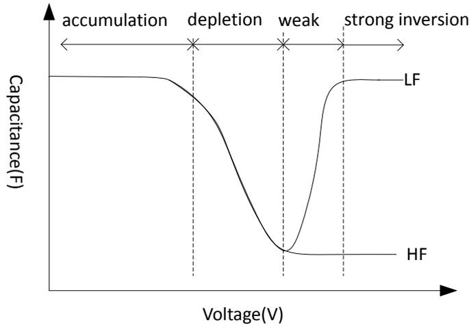
Figure 4.1 Ideal high frequency and low frequency Capacitance-Voltage curves<sup>37</sup>
