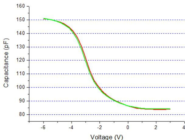
Figure 4.19 Detection of mobile charges in the oxide film
