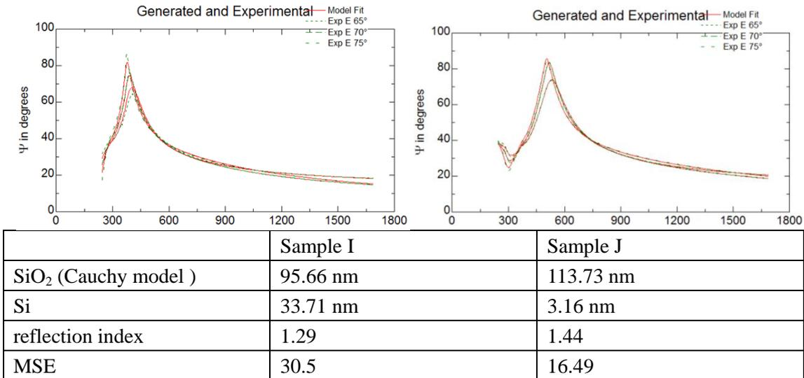
Figure 3.13 Ellipsometer results of the films bake at different temperature in the open air
