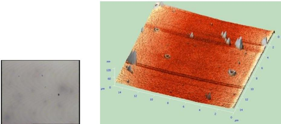
Figure 3.5 AFM result regarding the morphology of the solution processed SiO<sub>2</sub> film surface
