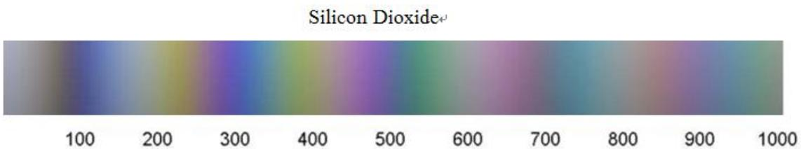
Figure 3.2 Reference color for SiO<sub>2</sub> films corresponds to film thickness in nanometers<sup>29</sup>
