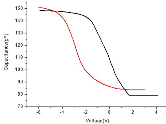
Figure 4.16 Comparison of theoretical and experimental HFCV.
