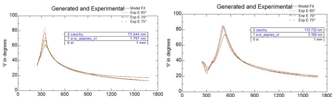
Figure 3.7 Ellipsometer measurement results of a brown part (left) and a blue part (right) on the film
