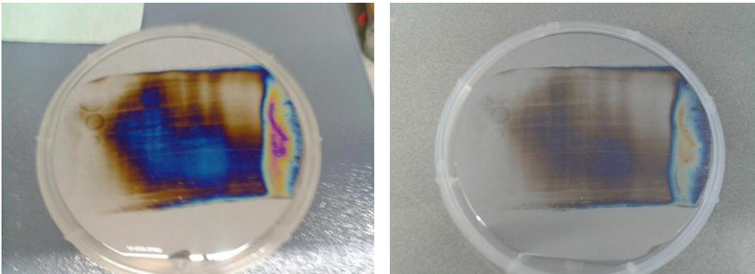
Figure 3.3 Comparison of film colors before and after oxidation
