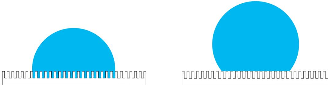
Figure 2.2 Wenzel model (left) and Cassie-baxter model (right) describing the influence of the surface roughness on the wetting level<sup>24</sup>
