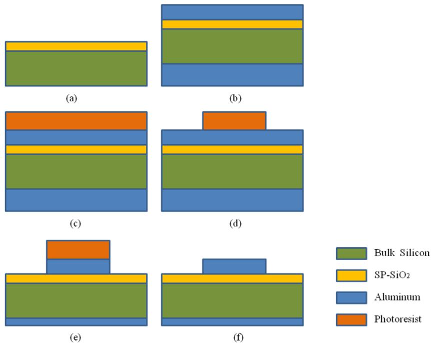
Figure 4.9 MOS-C fabrication procedures
