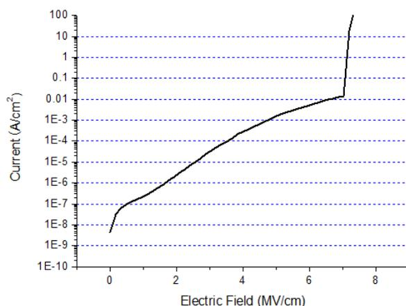
Figure 4.20 IV curve of the device fabricated in 400 °C
