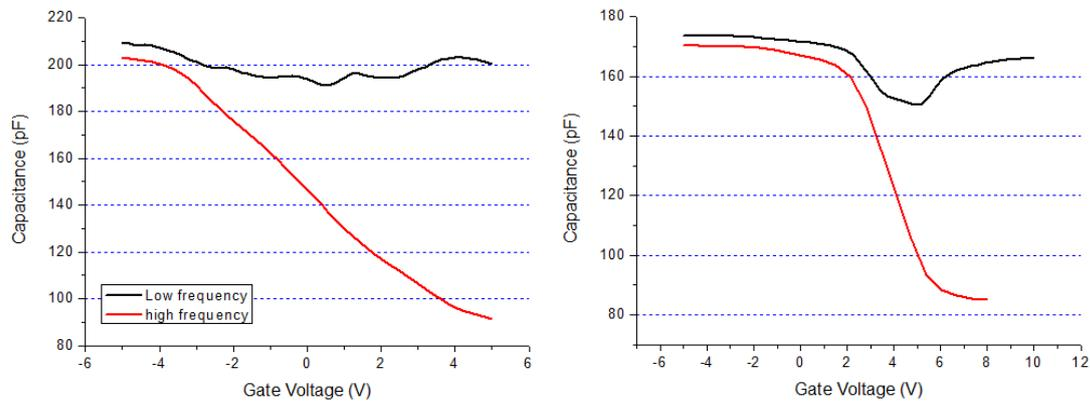
Figure 4.14 HF and LVCV of Sample K showing the improvement before (left) and after (right) postmetallization annealing
