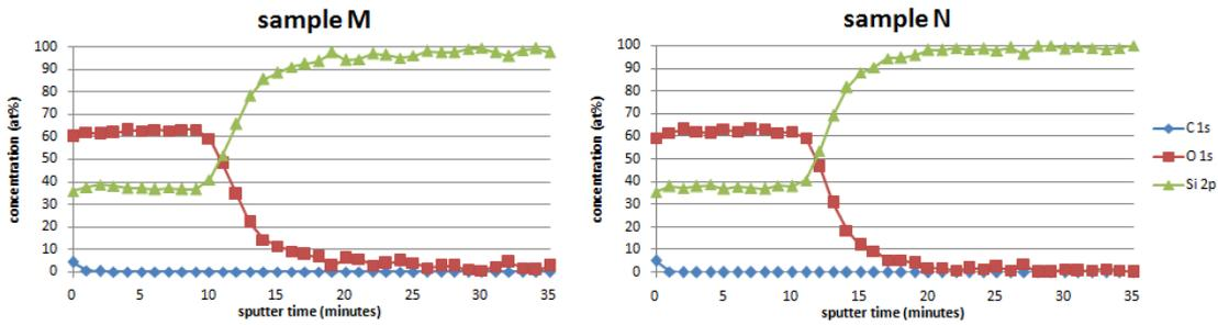
Figure 5.2 Results of the atomic concentrations in depth profile. Left: sample M, Right: sample N
