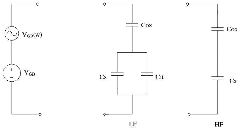
Figure 4.2 Equivalent circuit of applied gate voltage and MOS capacitor in low and high frequencies.<sup>38</sup>
