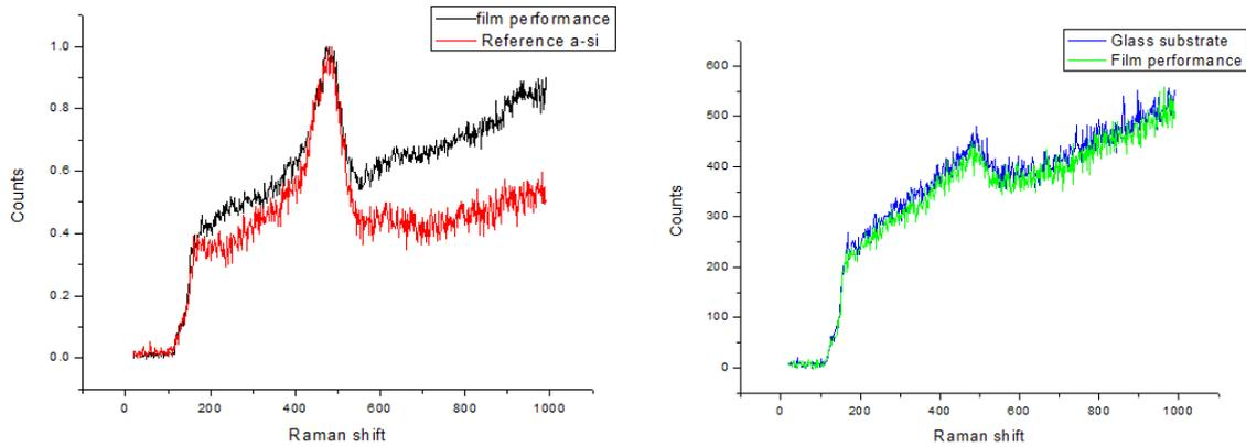
Figure 3.6 The Raman spectrum of the thicker part on the solution processed film compared to the reference amorphous silicon spectrum (left). The Raman spectrum of the thinner part of the solution processed film compared to the spectrum of bare glass substrate (right).
