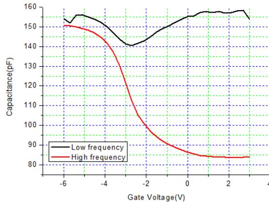
Figure 4.15 HF and LHCV of Sample L after postoxidation annealing
