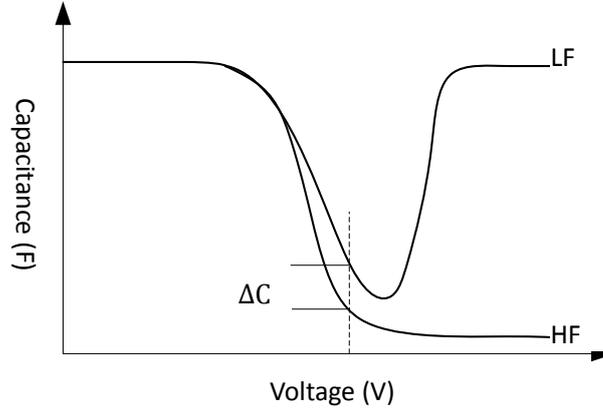
Figure 4.3 CV curve of MOS-C when considering the influence of interface states
