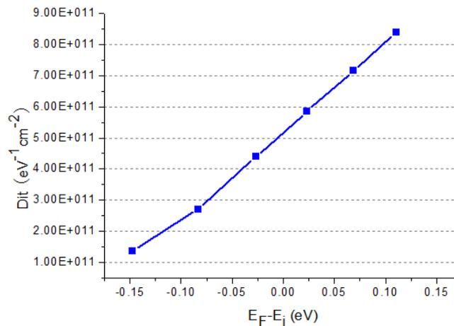
Figure 4.18 Interface state density as a function of silicon band gap energy
