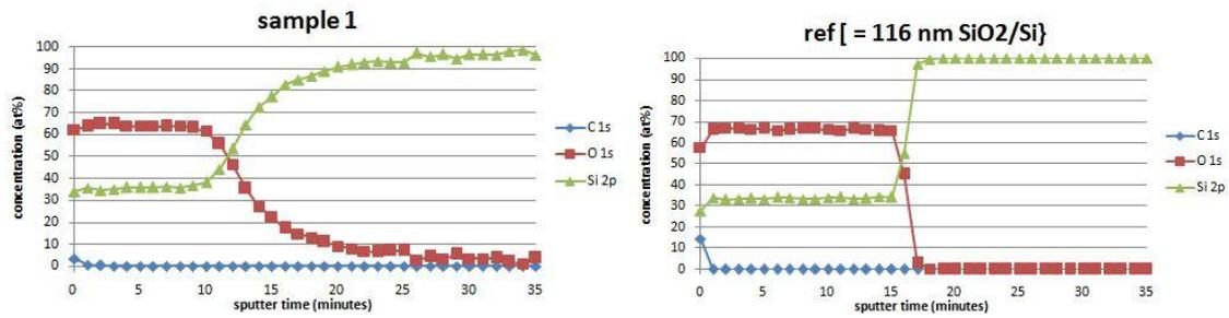
Figure 3.8 Results of the atomic concentrations in depth profile. Left: SP-SiO<sub>2</sub> sample with oxidation temperature of 400 °C, Right: thermal oxide reference sample
