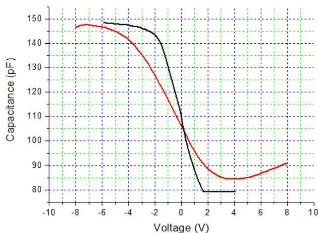
Figure 5.3 HFCV of solution processed film (red) and theoretical curve (black)
