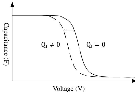
Figure 4.5 HFCV of MOS-C showing the influences of fixed oxide charges<sup>37</sup>
