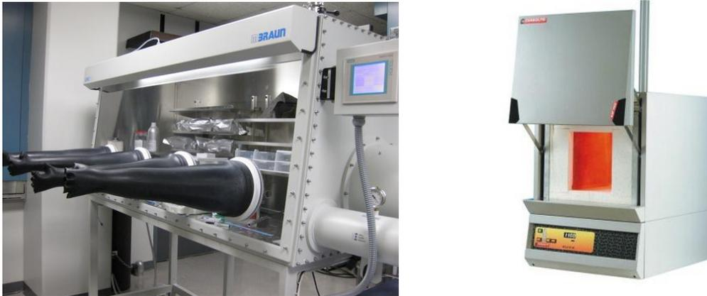
Figure 3.1 Mbraun Glovebox(left) and Carbolite Furnace(right)<sup>2728</sup>
