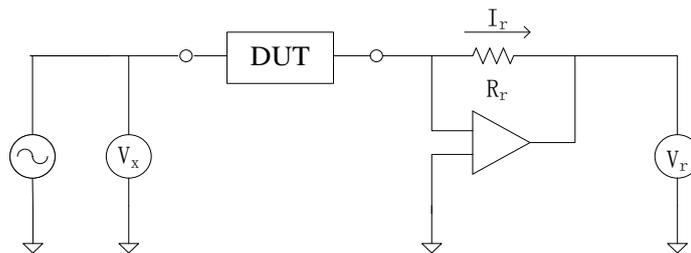
Figure 4.11 Working mechanism of LCR meter
