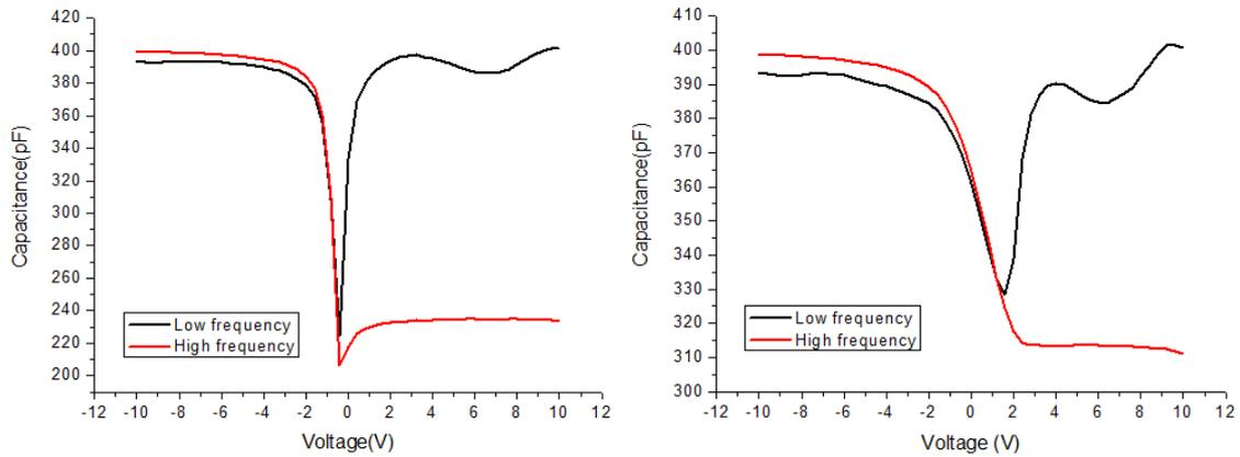
Figure 4.8 HF and LFCV of MOS-C with different substrate silicon resistivity. Left: 1-5  $\Omega\text{cm}$ , Right: 0.1-0.2 $\Omega\text{cm}$
