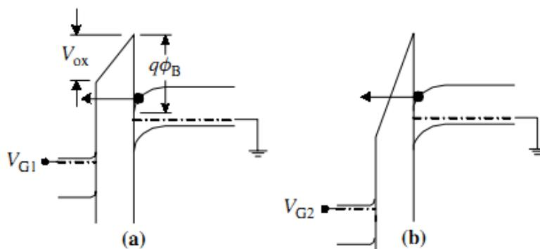
Figure 4.7 Band diagram of different tunneling mechanisms<sup>39</sup>
