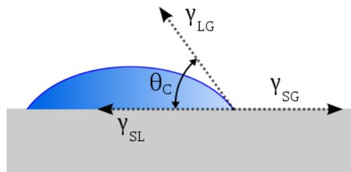
Figure 2.1 Schematic of the contact angle<sup>24</sup>
