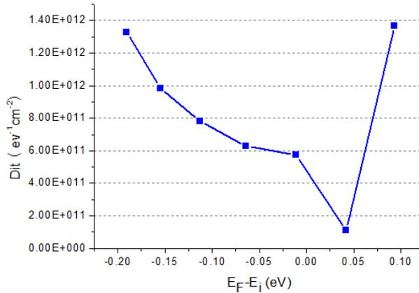
Figure 5.4 Interface trap density as a function of band gap energy
