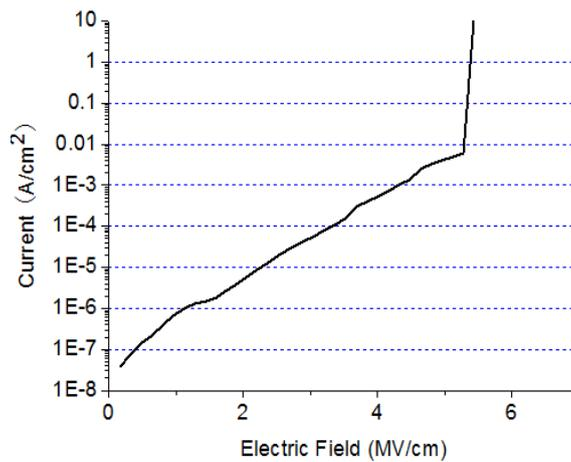
Figure 5.5 IV characteristics of liquid silicon processed film prepared at 350 °C
