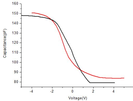
Figure 4.17 HFCV after shifting of the experimental curve
