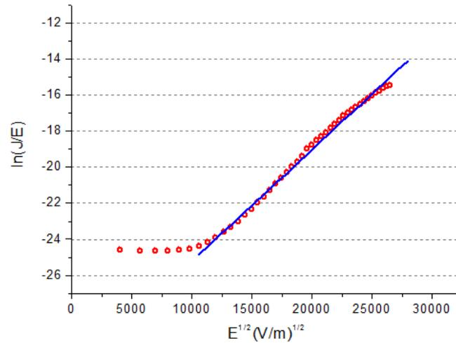
Figure 4.21 Linear fitting of IV characteristics using Frenkel-Poole model
