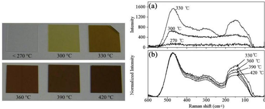
Figure 2.3 Photographic image of solution processed silicon films (left), Raman spectra of SP-Si films prepared in different annealing temperature.<sup>23</sup>
