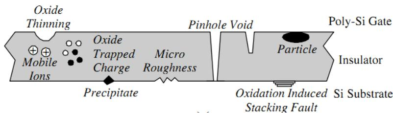
Figure 4.6 Schematic of the defects in the insulator.<sup>39</sup>
