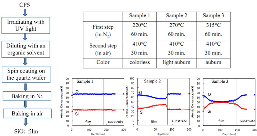
Figure 2.4 Fabrication steps, baking conditions and XPS results of SiO<sub>2</sub> films made by H. Tanaka<sup>13</sup>
