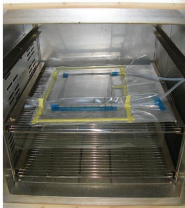
**Figure 4.5:** Position of vacuum bagged mould in the oven.
