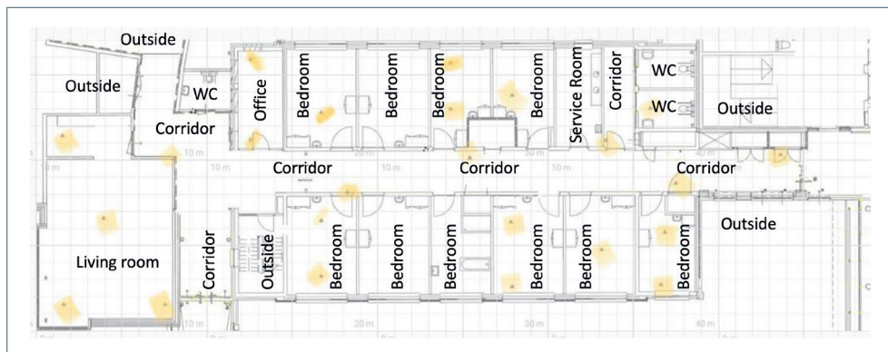
Figure 3. The set-up of location data collection in the ward (the locations of the sensors are marked yellow on the map, and the data collected is sent to the server in the Office via Wi-Fi gateways).
