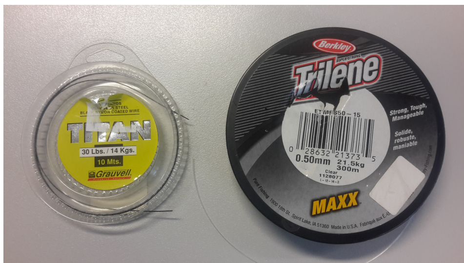
Figure A.19: Photograph of used wiring. The left wire is used for the mass. The right wire is used for the loadcell.
