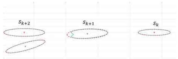
Fig. 2: Uncertainty ellipses for the purple vehicle of Fig.1 under two motion policies.  $\mathbf{s}_k, \mathbf{s}_{k+1}, \mathbf{s}_{k+2}$  are the estimated multi-modal position distributions for a given safety level. If the distributions overlap ( $\mathbf{s}_{k+1}$ ), the minimal area-enclosing ellipse (dash-red) is computed. Otherwise, the level set of each independent Gaussian distribution (solid cyan) is used.
