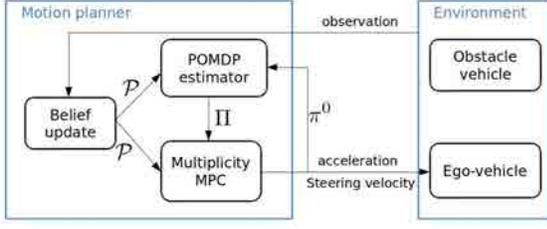
Fig. 3: Schema of the proposed method for joint behavior prediction and planning.  $\mathcal{P} = [\mathcal{P}^1, \dots, \mathcal{P}^n]$  are the belief weights of each obstacle vehicle and motion intention.  $\Pi = [\Pi^1, \dots, \Pi^n]$  are the estimated trajectories for each obstacle vehicle under all possible motion intentions. And  $\pi^0$  is the planned trajectory for the ego-vehicle.
