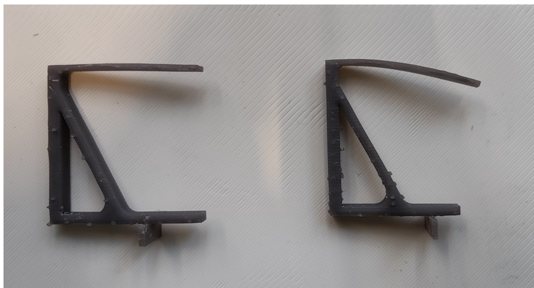
Figure 6.6: Effect of creep due to continuous loading over a month (left one is the unused piece, right one is the deformed piece after a month)
