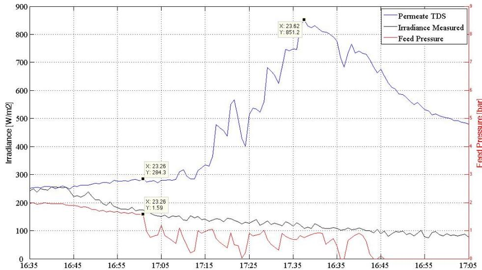
Figure 9.13: A closer look at the permeate TDS, Irradiance measured and feed pressure during shutdown.
