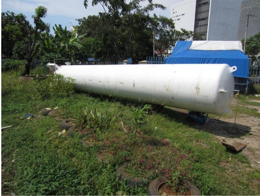
Figure 7.9: Hydro-pneumatic Storage Vessel
