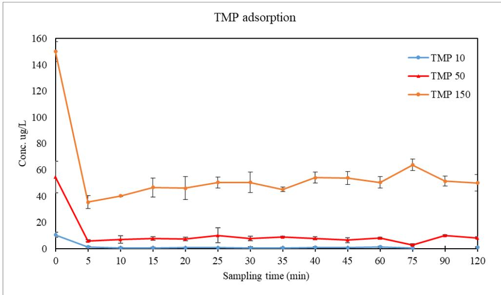
Figure 29 Adsorption of TMP at 37°C
