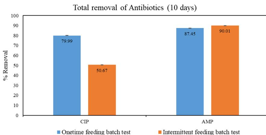
Figure 16 Removal efficiencies of CIP and AMP in two batch tests
