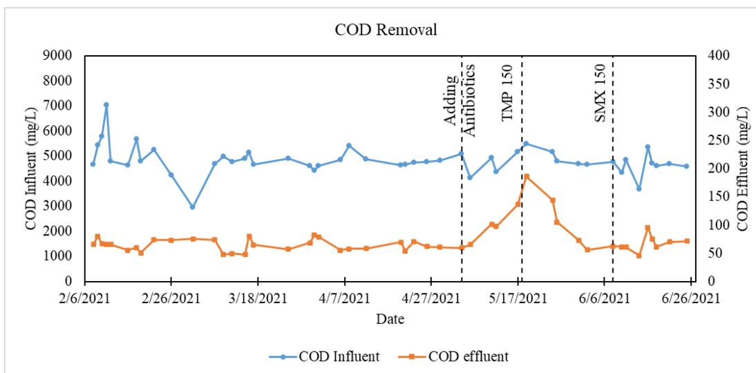
Figure 6 Removal of COD in reactor
