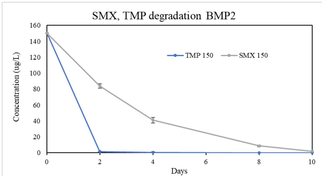
Figure 28 Degradation of SMX and TMP via intermittent feeding batch tests
