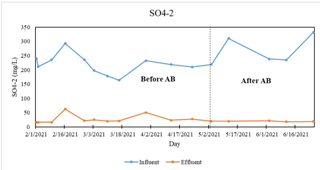
Figure 24 Removal of sulphate in reactor
