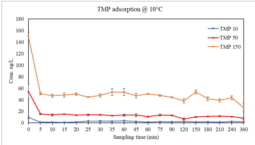
Figure 25 Adsorption of TMP at 10°C
