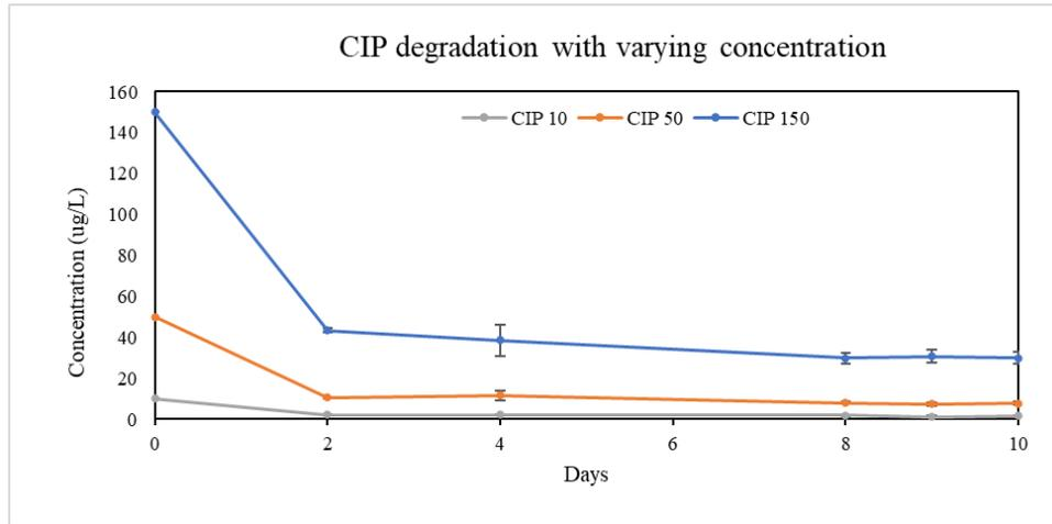
Figure 30 Removal CIP at varying concentrations in BD test 1
