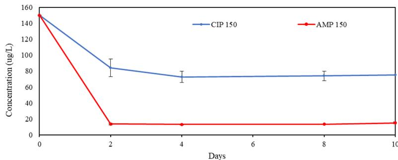
Figure 33 Removal of CIP and AMP in intermittent feeding batch tests
