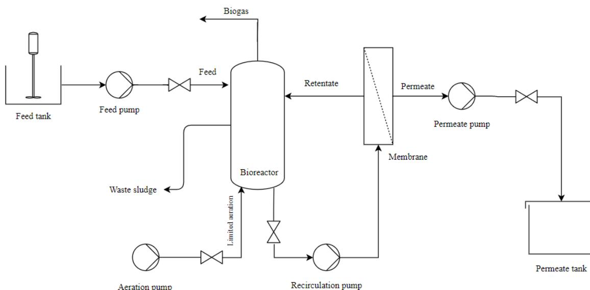
Figure 4 Piping and Instrumentation diagram of AnMBR
