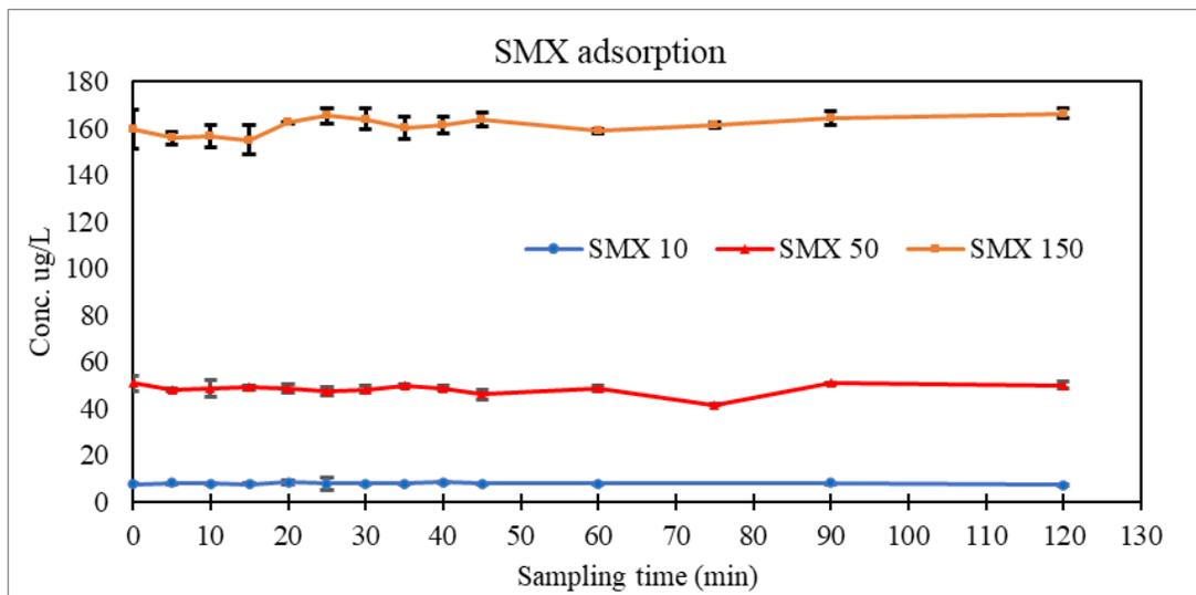
Figure 27 Adsorption of SMX at 37°C
