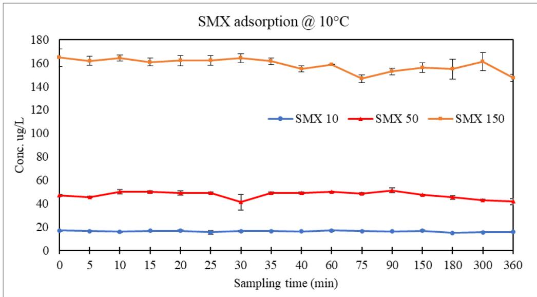
Figure 26 Adsorption of SMX at 10°C
