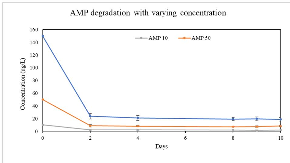
Figure 31 Removal AMP at varying concentrations in BD test 1
