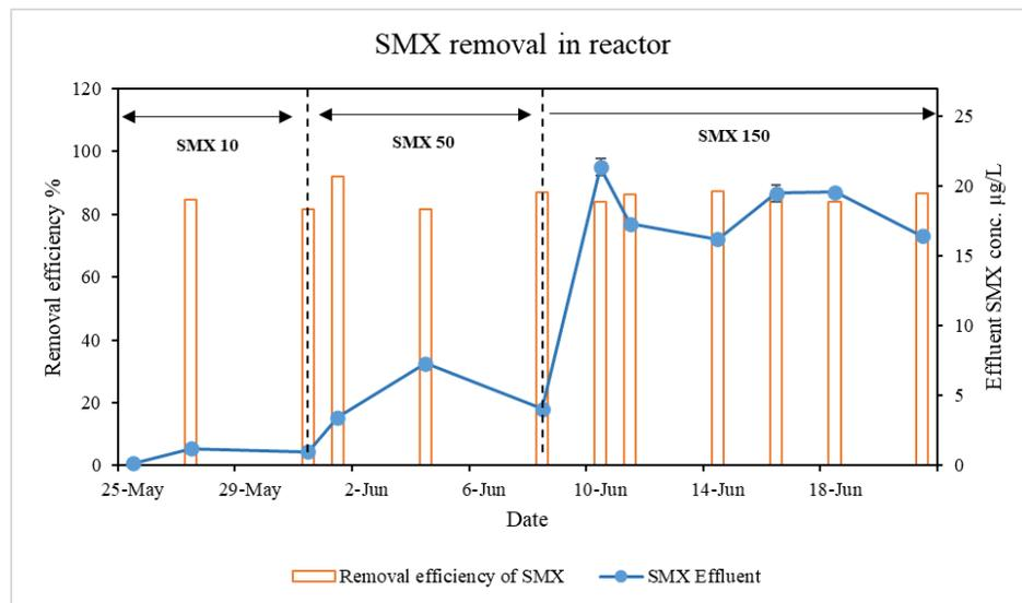
Figure 9 Removal of SMX in reactor
