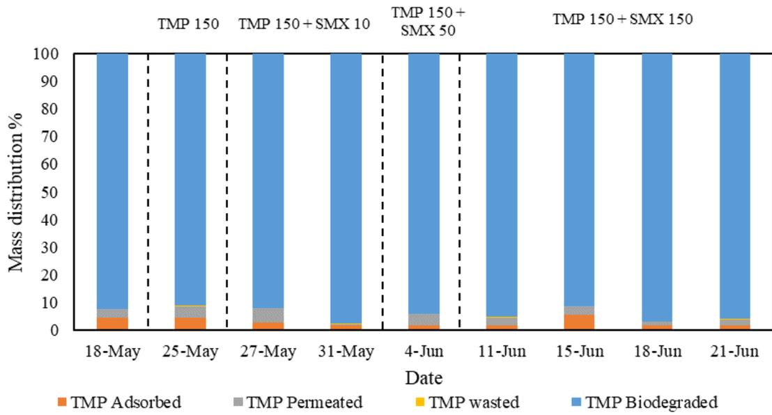
Figure 10 Mass balance of TMP in reactor
