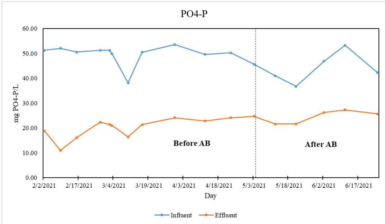
Figure 22 Removal of phosphate in reactor
