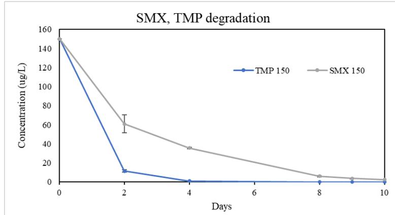
Figure 12 Removal of SMX, TMP through degradation tests with one-time feeding
