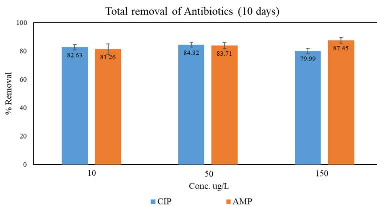
Figure 15 Removal of CIP and AMP at different concentrations
