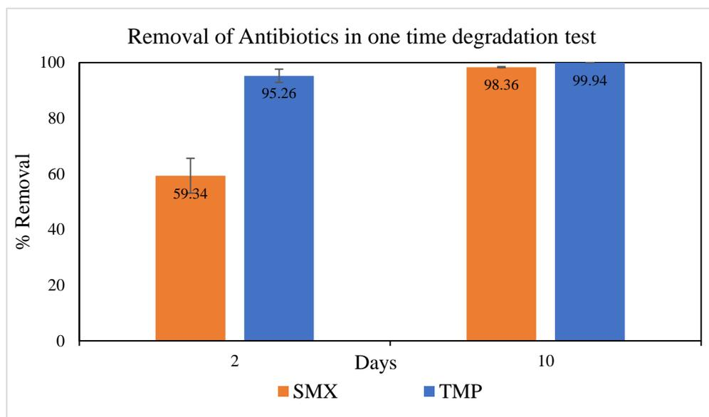
Figure 17 Removal of SMX and TMP in 2 and 10 days of biodegradation test with onetime feeding
