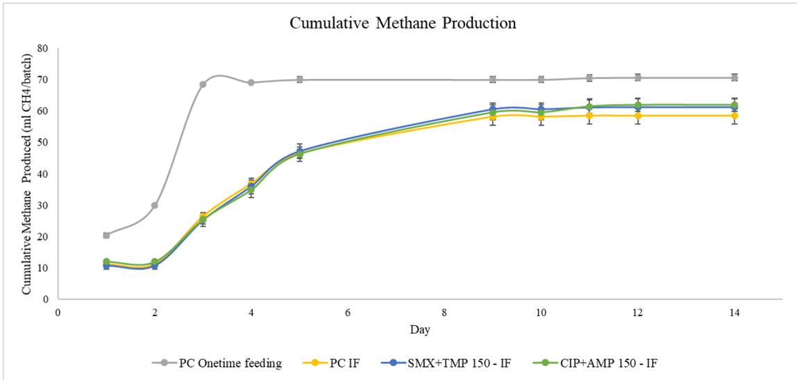
Figure 32 Cumulative methane production in intermittent feeding batch test
