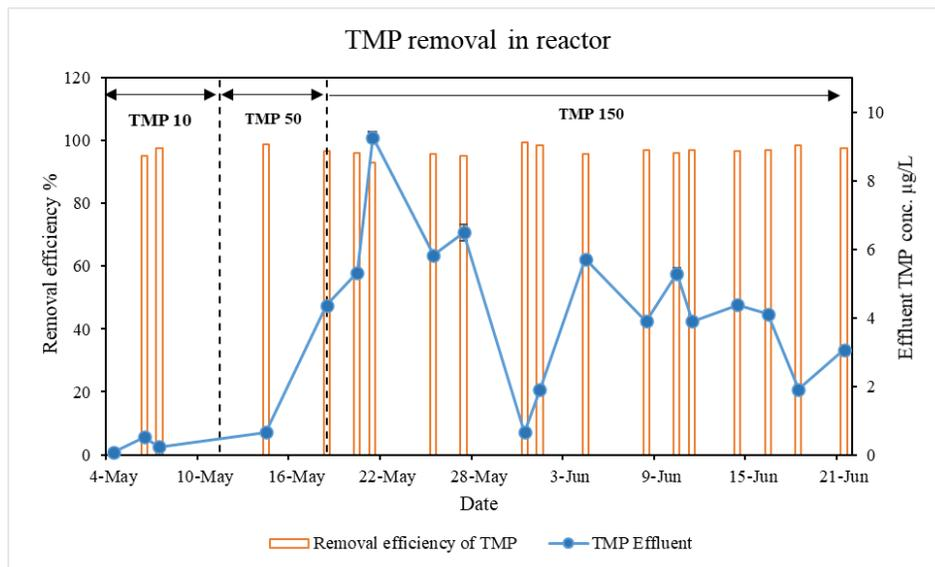
Figure 8 Removal of TMP in reactor
