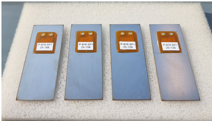
Figure D.4: Flexures with bonded Piezoelectric Transducers
