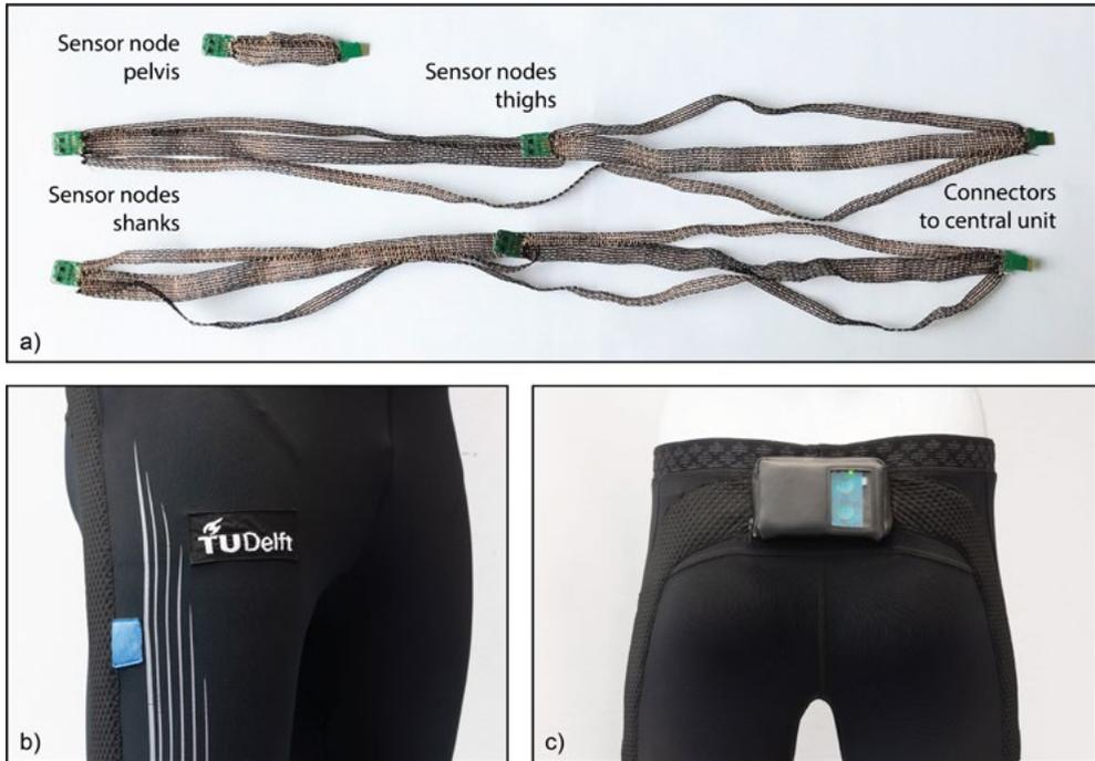
Figure 10.3. a) The sensor module assembly. b) Detail of the sensor tights: the sensor of the right thigh is covered with a blue textile. c) Central unit of prototype 4.
