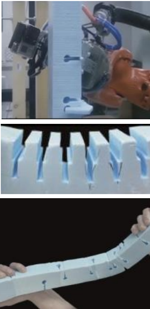
Figure 5. Materialization experiments and robotic production process involve robotic milling (top), preliminary research on the geometry of the milled section (middle) and robotically fabricated component (bottom)
