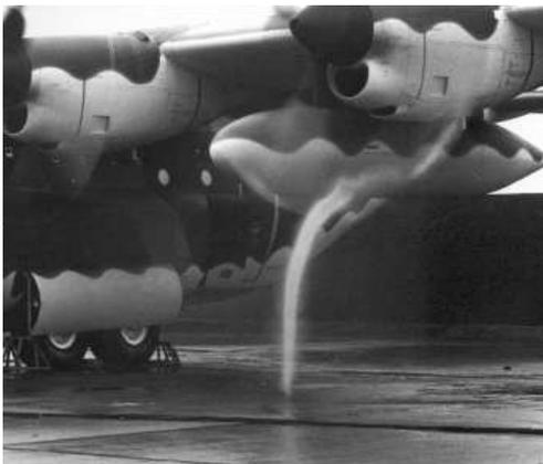
(a) Ground vortices toward the propeller of C130 aircraft<sup>[1]</sup>
