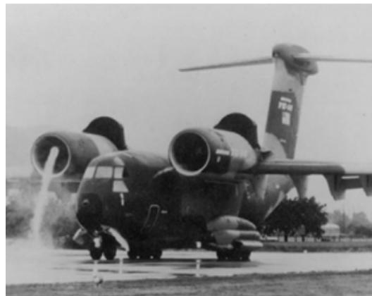
(b) Ground vortices toward the engine inlet on a YC-14 aircraft<sup>[1]</sup>
