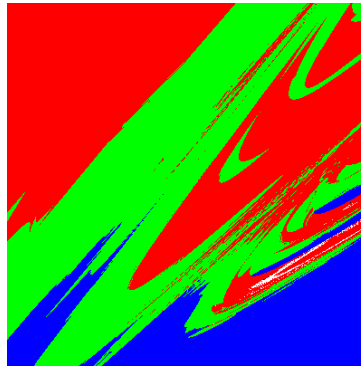
Fig. 10. Basins of attraction for a seven-dimensional Double Gauss optimization problem. The initial curvature of the first surface is plotted vertically, and the initial curvature of the second surface is plotted horizontally.
