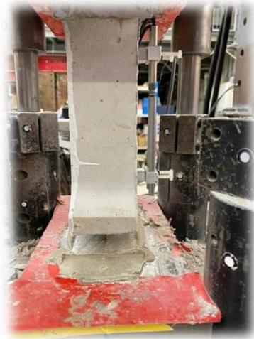
Fig. 5.60: Failure of SHCC-glue interface in tensile test
