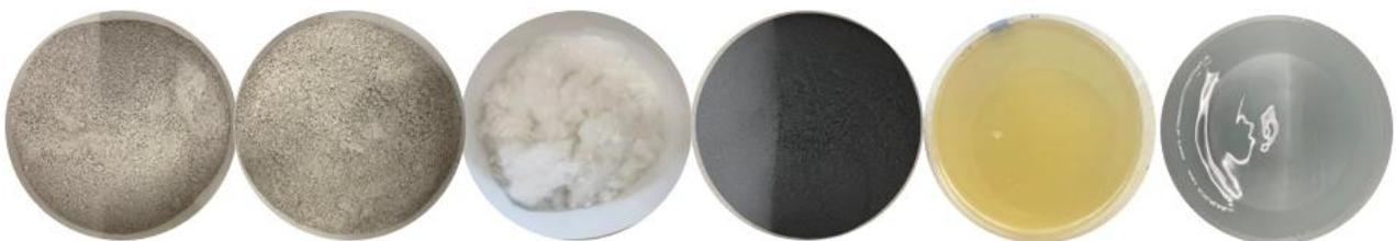
Fig. 3.10: Ingredients used in PVA-SHCC. From left to right: CEM III/B, limestone, PE fibers, silica fume, superplasticizer and water
