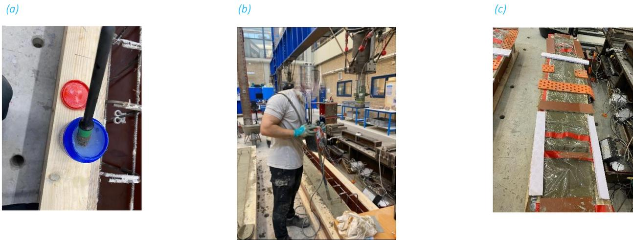
Fig. 4.5: (a) Vaseline used on top of profiled interface (b) Vibration needle used to vibrate CC layer (c) Beam molds covered after CC layer casting
