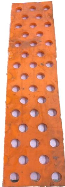
Fig. A. 2: Silicon mold used to construct profiled interface
