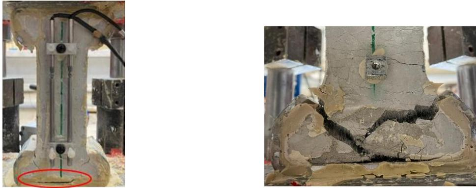
Fig. 5.64: SHCC detaching from steel hand (at its flat part) (left) and SHCC failure outside gauge area (right)
