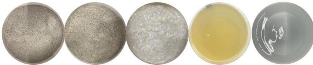
Fig. 3.9: Ingredients used in PVA-SHCC. From left to right: CEM III/B, limestone, PVA fibers, superplasticizer and water
