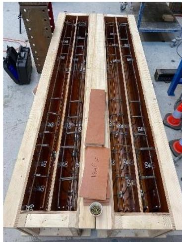
Fig. 4.3: *Wooden molds used to cast the beams*
