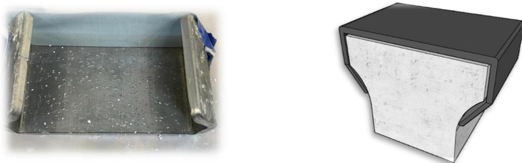
Fig. 5.63: Steel hand used in series 2 (left) and sketch of dogbone glued in the steel hand (right)
