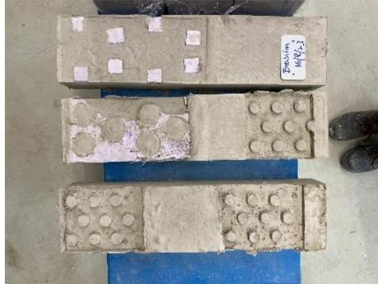
Fig. 4.2: *Profiled interfaces after demolding*
