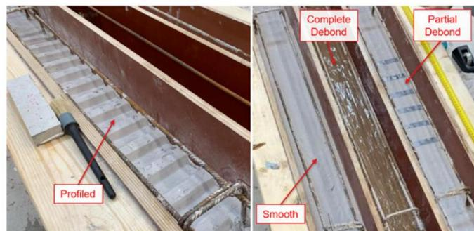
Fig. 2.23: Photos of interface conditions as realized by [52]
