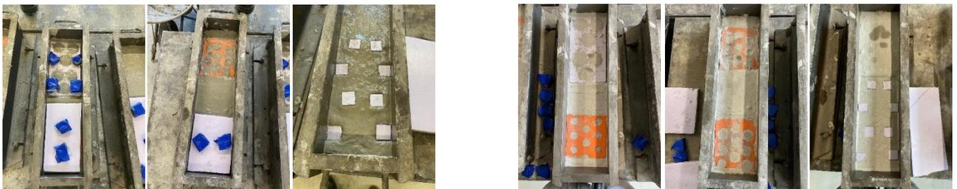
Fig. 4.1: Fresh (left) and hardened (right) state of profiled interfaces
