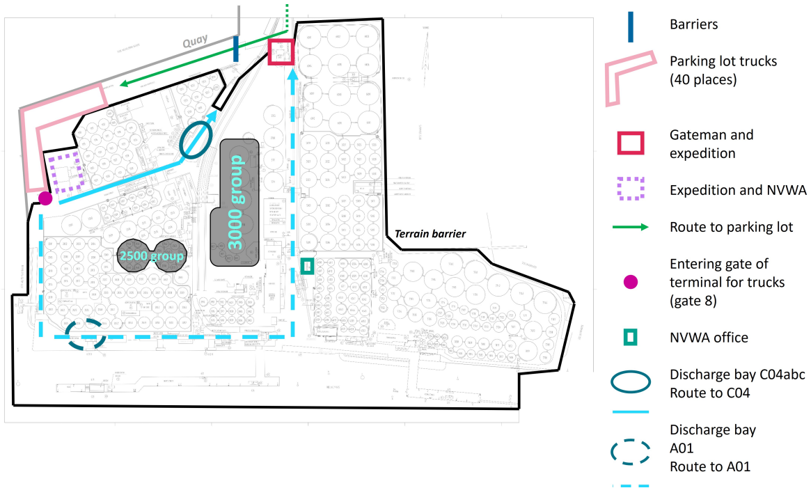
Figure 4.3: Map of Vopak Terminal Vlaardingen with important truck logistic indicators. Truck Arrival Management System: Complementary Truck Arrival Management System
