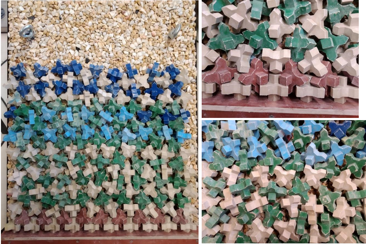
Figure 3.19: Overview of the Xbloc®s on the slope
