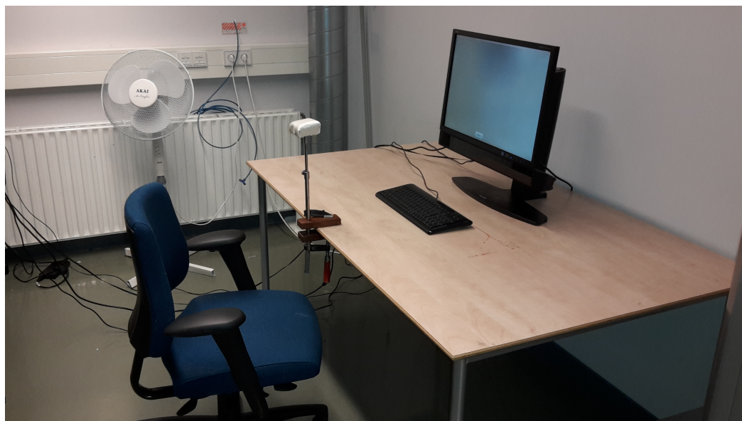
Figure 1 Experimental equipment: monitor with built-in eye tracker (SmartEye DR120), chin-rest, and keyboard.
