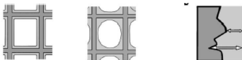
Figure 7. Schematic representation of actual layer thickness compared to a uniform film layer (left); thicker film in monolith channel corners due to surface tension (middle); thicker gel layer due to uneven surface (right).
