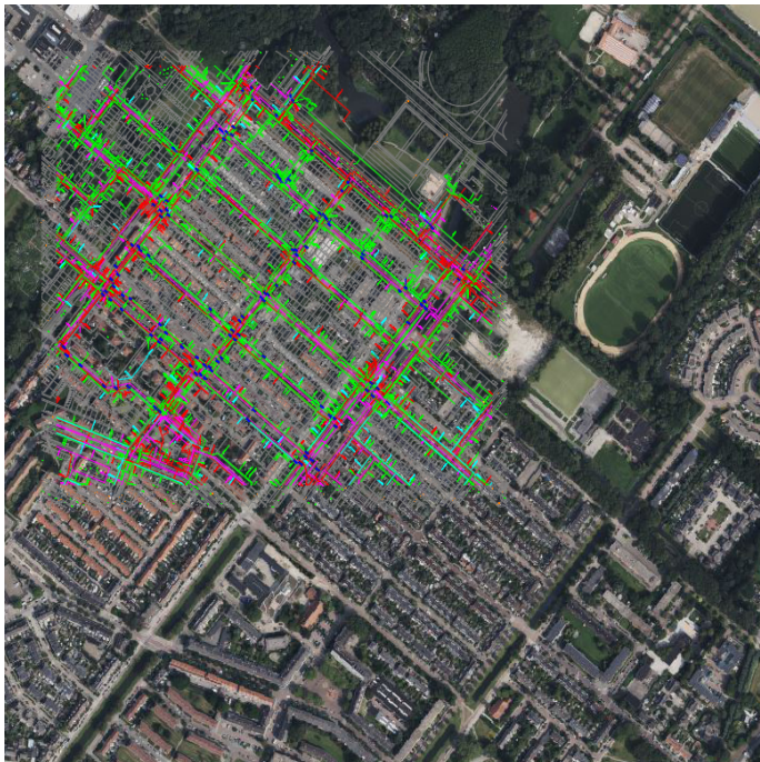
Figure 6.5: Incorrectly geo-referenced Rotterdam data
