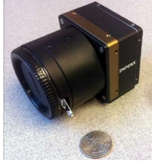
Figure 3 Photograph of prototype plenoptic camera.
