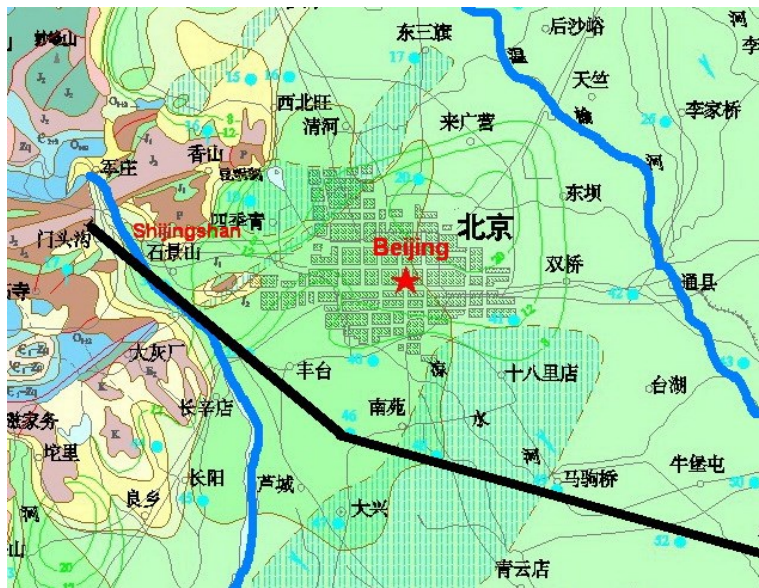
Figure 4-16 Hydrogeological map of Beijing area. Intercept from full map. Black line represents cross section location and blue line represents river and red spot represents city location with name in black and red line represents edge of unit.
