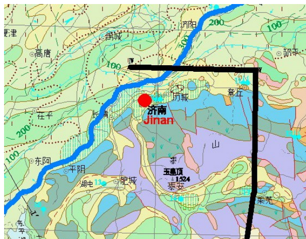
Figure 4-20 Hydrogeological map of Jinan area. Intercept from full map. Black line represents cross section location and blue line represents river and red spot represents city location with name in black and red line represents edge of unit.
