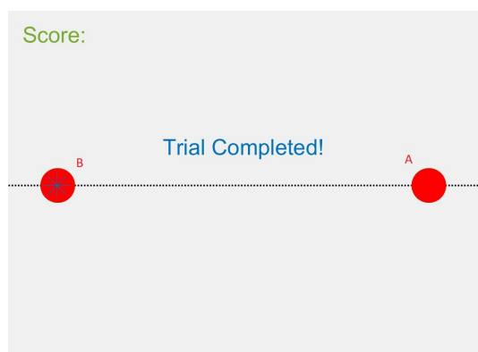
Figure 2: Final design of the visual environment used. The participant was instructed to move from circle A to B before and after a hold period of 5s . A cursor is currently placed in circle B, which represents the position of the handle and moves with user input. The position cursor only moved in the horizontal direction visualizing the flexion and extension of the wrist.
