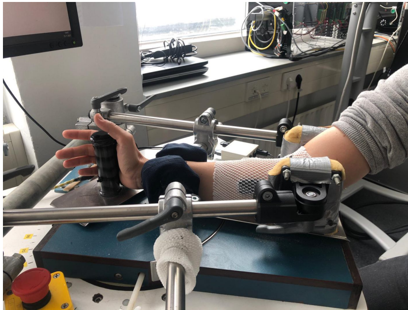
Figure 18: The PoPe setup in real life. During the experiments, the subjects were instructed to keep the hand relaxed and open.
