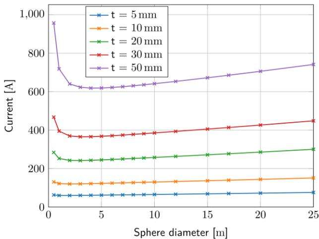
Fig. 6. The analytical solution is used to plot the optimum degaussing current as a function of the size of the object with a relative permeability of  $\mu_r = 100$ , for several different wall thicknesses.
