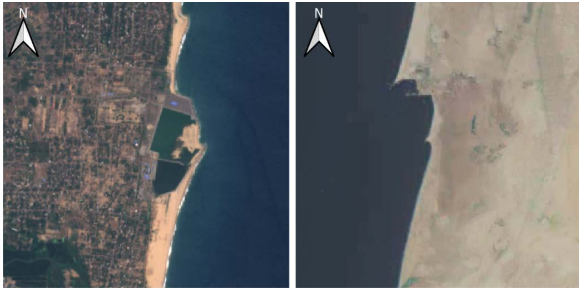
Figure 2.24: Left: Harbour siltation, Oluvil Port, Sri Lanka; right: updrift accretion, downdrift erosion, Port of Nouakchott, Mauretania. Images from Sentinel-2 cloudless by EOX IT Services GmbH are licensed under CC BY 4.0.
