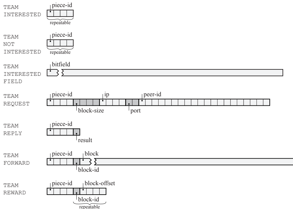
Figure A.2: The messages and their payload used by the Light Supervised Teaming protocol.
