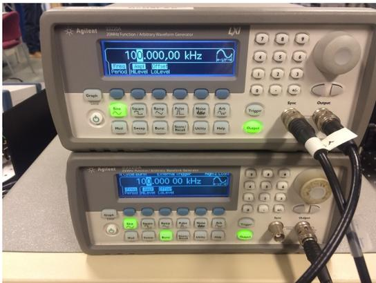
Figure 2.21: Photograph of the master and slave function generator and their output connections
