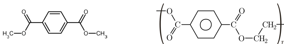
Figure 3.2 Chemical structure of di-methyl terephthalate (DMT, left) and polyethylene terephthalate (PET, right)
