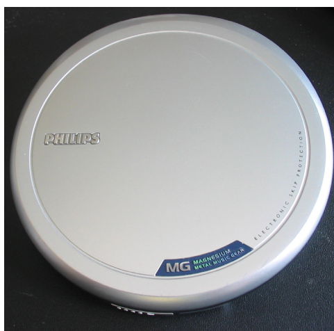
Figure 2.2 Philips AX7201 portable CD player with diecast magnesium lid.
