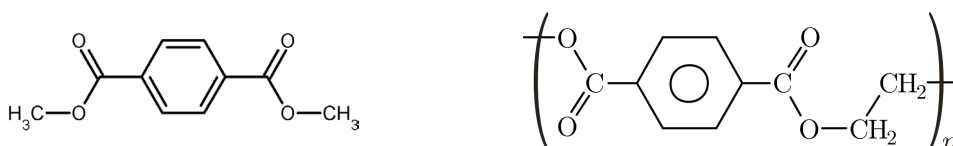
Figure 6.1 Chemical structure of di-methyl terephthalate (DMT, left) and polyethylene terephthalate (PET, right).
