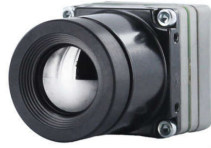
Figure 10.44: FLIR Quark 640 with 6.3 mm lens, mass: 18.3 g, 1.0 W @ 30 fps, 22x22x12 mm, 640 × 512 pel [69]
