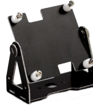
Figure 10.45: Fiberglass camera tilt mechanism, mass: 8 g, 42x40 mm [70]
