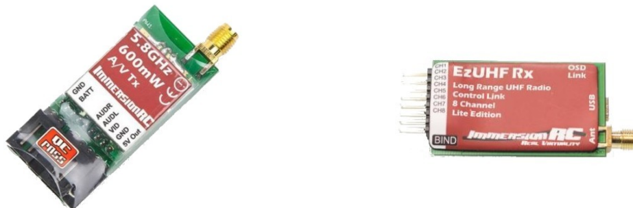
(a) EzUHF 5.8GHz 600mW Tx, mass=18g, 50 x 23 x 15 mm, 3 W
