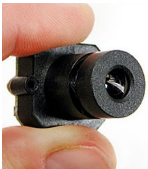
Figure 10.46: V-XA095-5V-PCB-3.6 Single Chip Color CMOS, mass: 2 g, max. 0.1 W @ 30 fps, 21 x 21 mm [71]
