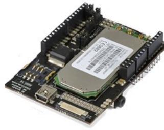
Figure 10.39: Cooking Hacks 4G cellular network shield, mass 27 g, avg. power 4 W, max. 8 W [64]
