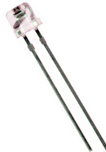
Figure 10.64: Photo-conductive resistor (<1 g) [98]
