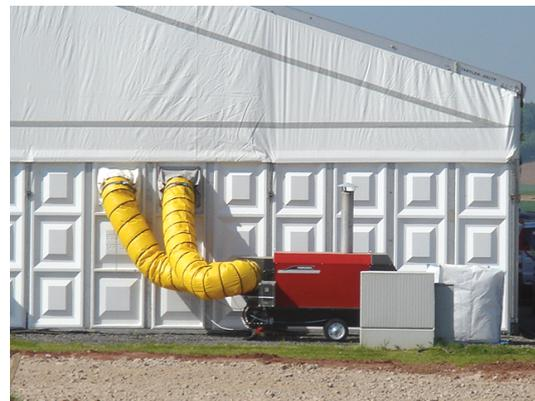
Figure 2.3: The mobile/movable system having multiple hoses is showcased. As can be seen, it has just 1 cavity on the left side through which just 2 hoses are connected. The system is placed outside the tent inside which a heating effect is needed.
