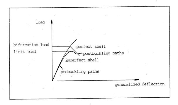
Fig. 1: Fundamental concepts in buckling analysis
