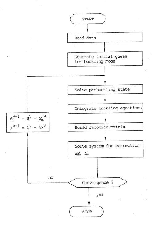
Fig. 5: Flow diagram of the computer program
