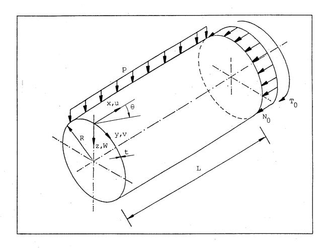
Fig. 2: Cylinder geometry and applied loading
