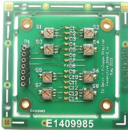
Figure 4.12: Designed PCB to implement variable capacitance.
