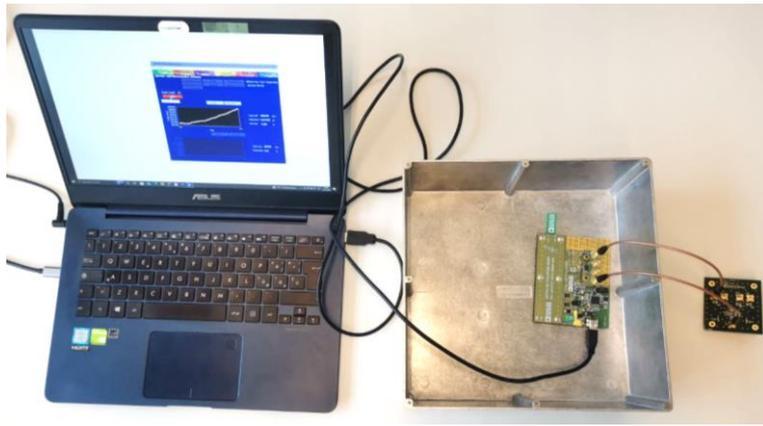
Figure 6.3: Measurement setup and connection for AD7746.
