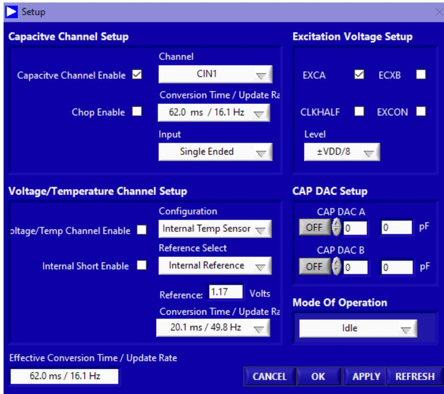
Figure D.3: AD7746 setup screen.
