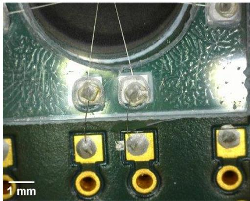
Figure 5.14: Investigated alternative to ultrasonic wire bonding.
