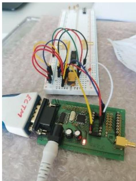
Figure 4.5: Setup for test of evaluation board compatibility.
