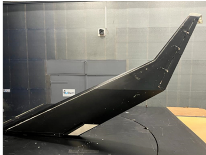
Figure 2.9: Bottom view of final flap design selection on OJF 4.8% scale Flying V model [4]
