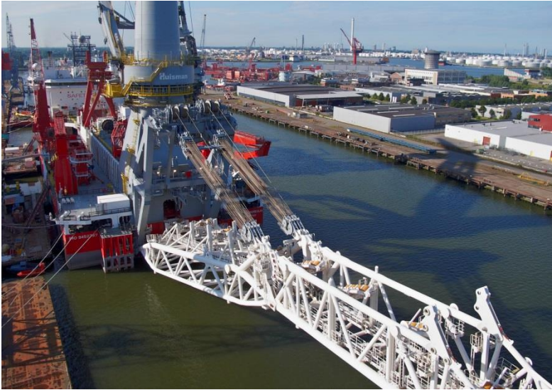
Figure 10-7: Stinger of Seven Borealis connect to the vessel transom
