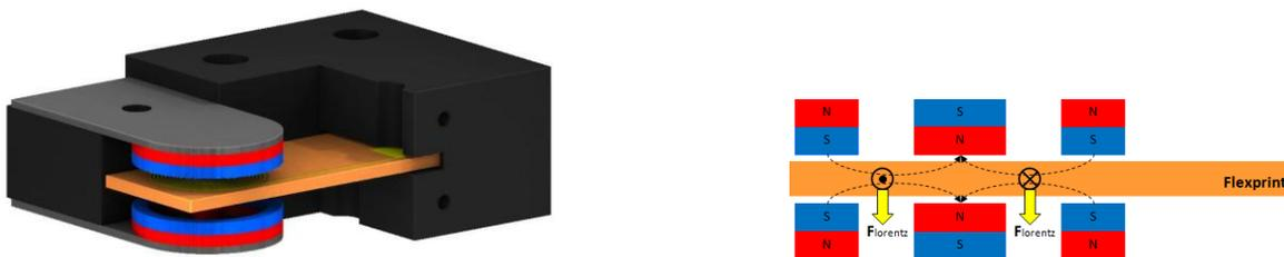
Figure 4. 1, left) the test sample: the flexprint with coil inside was suspended through a fabricated frame (black) which is additionally utilized to hold the magnets from an orthogonal direction; right) the corresponding driving mechanism.
