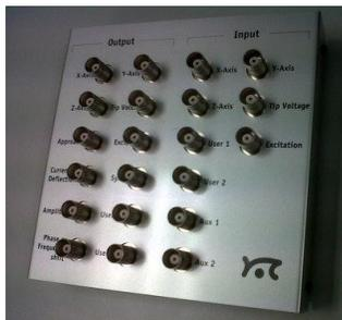
Figure 3. 6, the BNC breakout box from Nanite B
