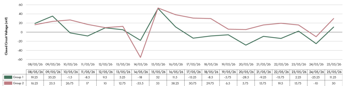
Figure 46: Average closed circuit voltage measurements for Groups 1 and 2 of the experiment.
