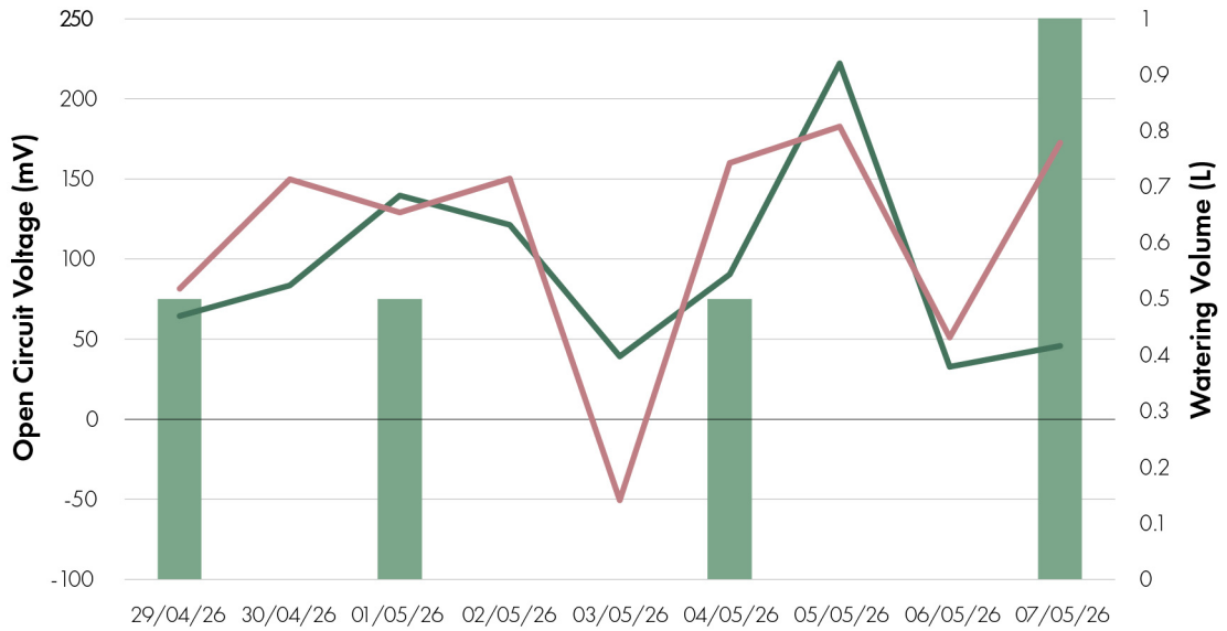
Figure 44: Comparison of average open circuit voltage measurements and watering schedule at the initial stage of the experiment.
