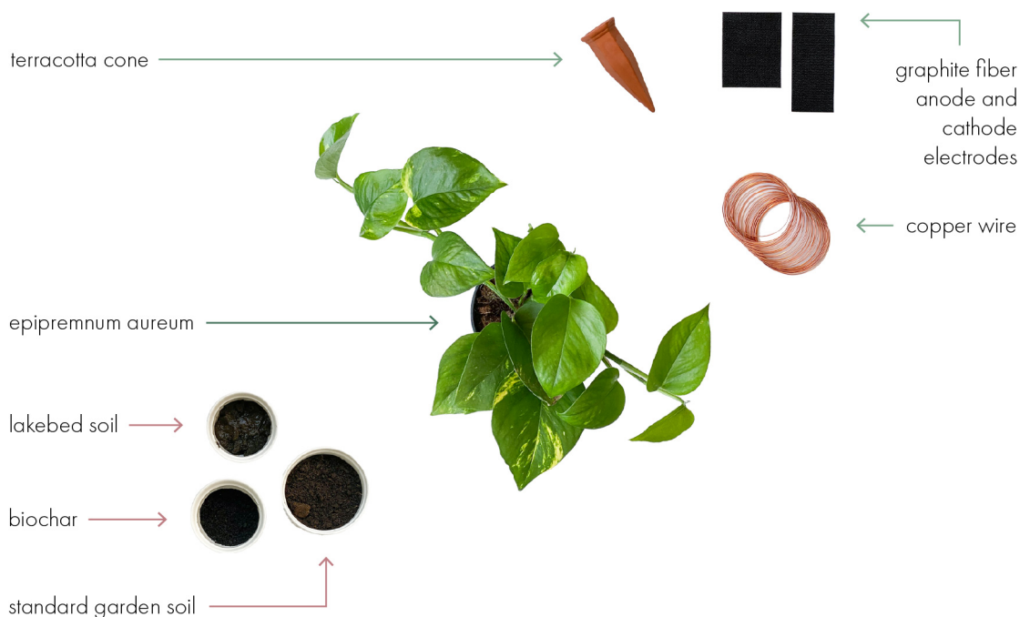
Figure 32: Materials of samples with PMFC reactors.
