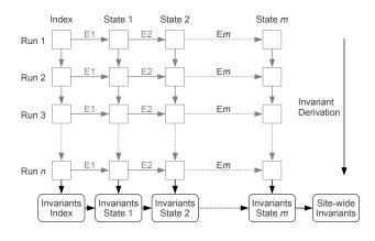
Figure 7: DOM invariant derivation across multiple states and execution runs.
