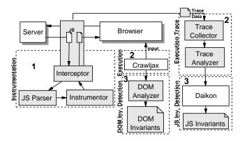
Figure 1: Processing view of our JavaScript and DOM invariant detection approach.
