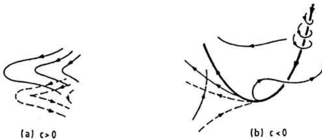
Fig. 5 Local flow structures near a cusp singularity in the skin friction field
