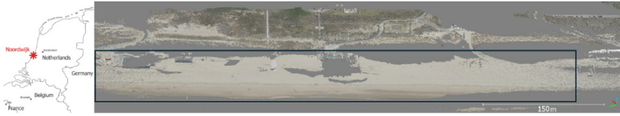
Fig. 1. Example of a point cloud of the beach at Noordwijk colored using aerial photography of the Dutch government (pdok/beeldmateriaal.nl). The black box indicates the area of the point cloud used for the analysis.
